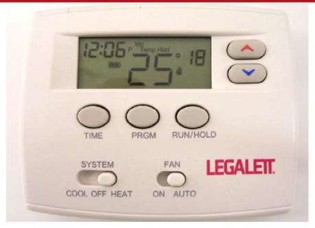
The main source of heat is the LEGALETT System. If there is a supplementary heat supply, such as radiators or air heating, the temperature setting for the latter should be approximately 1-2°C (2-4°F) lower than the setting for LEGALETT.
