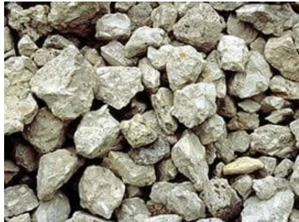
Recycled Concrete Aggregate. Photo Courtesy of Portland Cement
