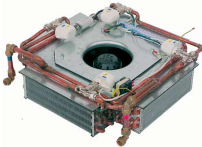
The 4000W heating unit is installed in the foundation slab or intermediate floor, and contains a fan and four water/air-exchangers, with valves that are controlled by 1
