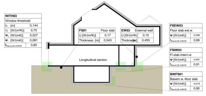
GEO-Passive Slab Foundation System - Type 2 | ID: 1550fs03
