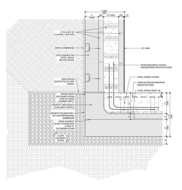
THERMALWALL PH PANEL DETAIL AT RAFT SLAB - SUBGRADE ICF WALL CONSTRUCTION
