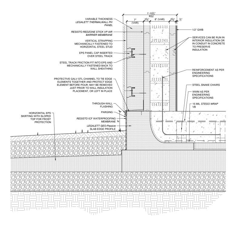
THERMALWALL PH PANEL DETAIL AT RAFT SLAB - AT GRADE ICF WALL CONSTRUCTION
