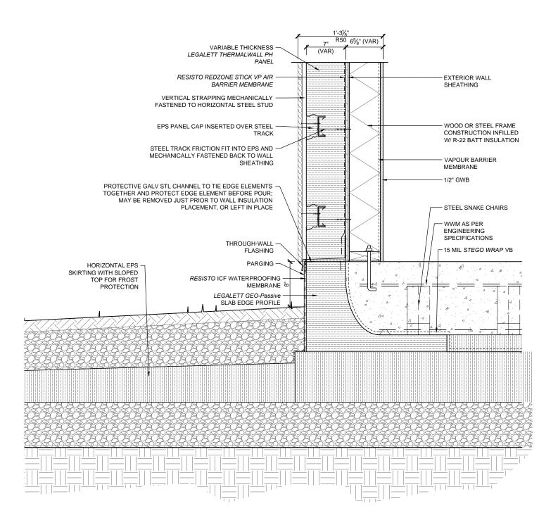
THERMALWALL PH PANEL DETAIL AT RAFT SLAB - AT GRADE FRAME WALL CONSTRUCTION
