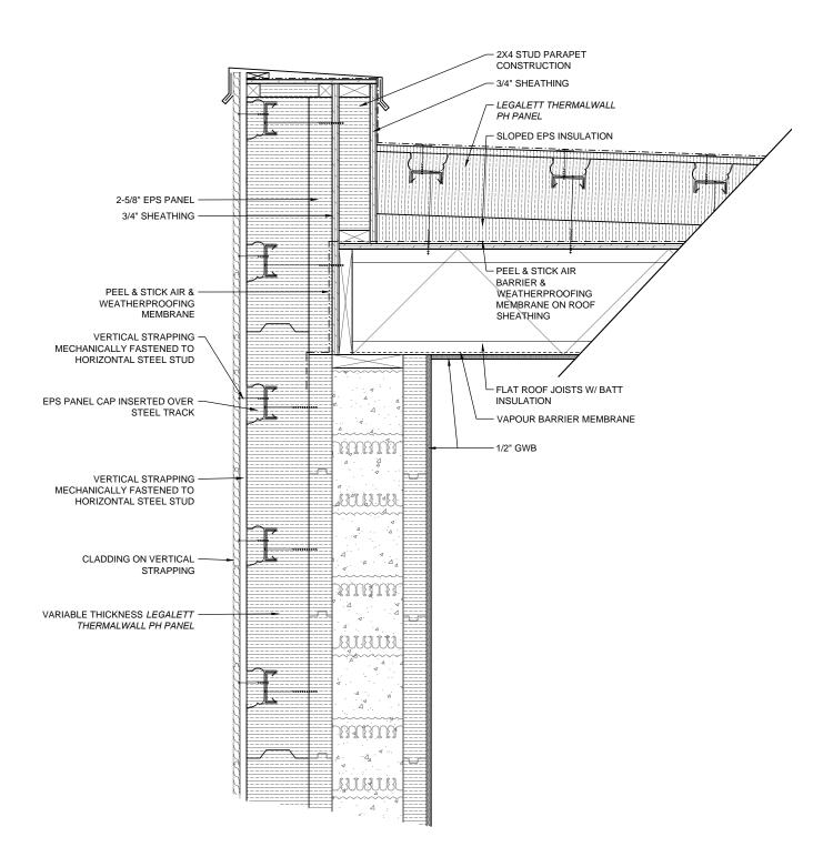
THERMALWALL PH PANEL DETAIL AT PARAPET / TJI ROOF CONSTRUCTION ICF WALL CONSTRUCTION
